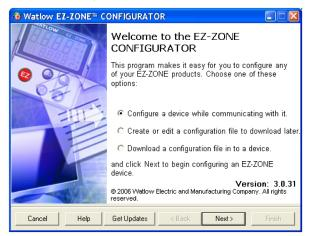
The EZ-ZONE configurator software is used to set up Watlow EZ-ZONE products in one simple process. It works without requiring the purchase of any communication options because it uses the standard bus communications protocol that is included with all EZ-ZONE products. EZ-ZONE configurator can be used for on-line and off-line configurations and downloading previously saved setups. It is available as a FREE download at www.watlow.com.
