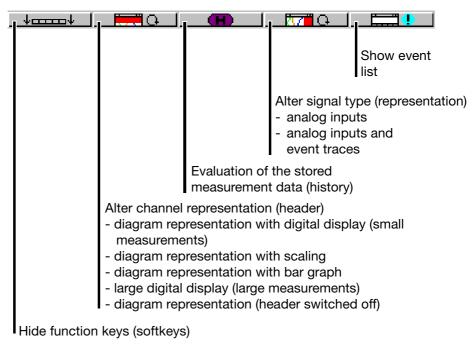
If the paperless recorder is equipped with "Counters/Integrators" (extra code), the symbol for indicating the counts will now appear below the softkey on the right, the symbol for showing the event list is shifted to the counter display.
