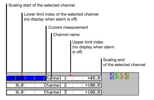
Use the parameter Parameterization  $\rightarrow$  Diagram view  $\rightarrow$  Channel indication to select which bar graph (from which channel) is to be displayed.
