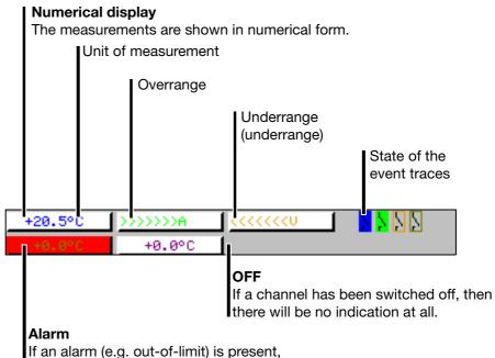
the measurement of the channel is shown on a red background.
