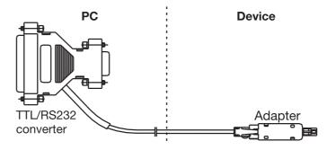
**Setup - USB** You will need the interface cable (including adapter) in this case. It is available as an accessory for the recorder.
