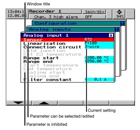
The configuration of the recorder is sub-divided into the following levels:
