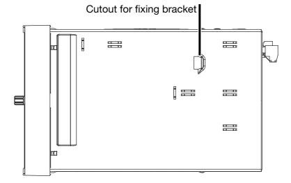
Push the fixing brackets up against the back of the panel and tighten them evenly.
