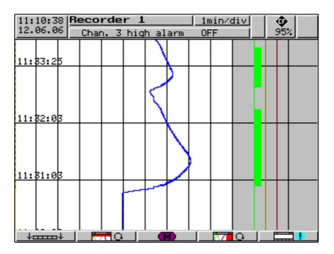
This display type is limited to the curve display.
