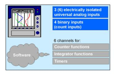
These are **not** electrical measurement inputs (hardware), but channels which are calculated by the paperless recorder (software).
