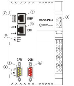
Figure 1: Interfaces varioPLC
