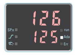
After successful self-tuning, the AdA-LED is off and the controller continues operating with the new control parameters.
