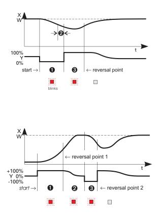
reversal point 2, parameters Pb2,  $k \cdot 2$ ,  $k \cdot d2$  and  $k \cdot 2$  are determined and the self-tuning attempt is finished. Control to set-point W is using the new parameters.
