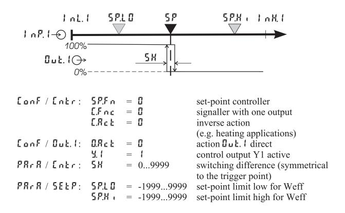
For direct signaller action, the controller action must be changed (LonF / LnEr / LReE = 1)
