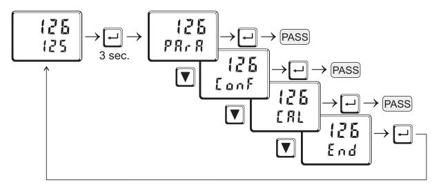
**PRrR** - level: At **PRrR** - level, the right decimal point of the upper display line is *lit continuously*.
