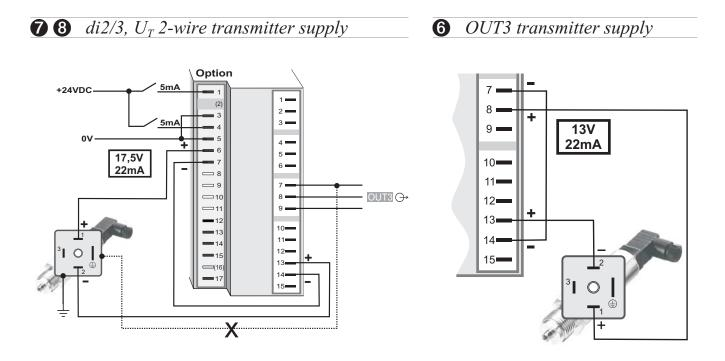
$\sum$  If U<sub>T</sub> and the universal output OUT3 is used there may be no external galvanic connection between measuring and output circuits!
