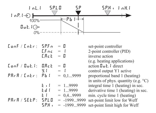
For direct action, the controller action must be changed (LonF / Lotr / L.Rct = 1).
